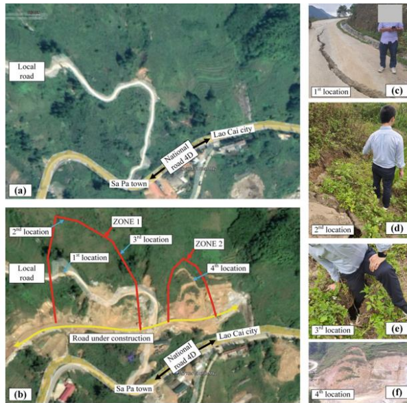
Fig. 3 Morphological changes of the slope by time and landslide views: a before road construction on October 30th, 2019; b during road construction on October 27th, 2020; c crack on local road 155; d crack on head scarf at zone 1; e crack along slide body at zone 1, and f head scarfs at different stages at zone 2
